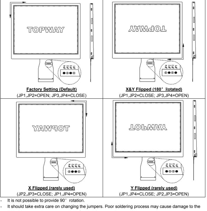
TFT. Disconnect the power supply before any jumper adjustment!
