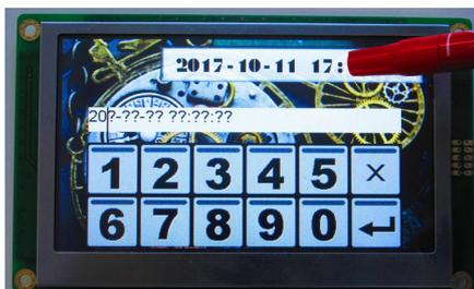
Touch the RTC area on the main page and pop up the PIP (RTC) key board
