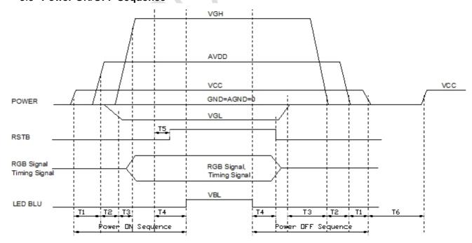
Note 1: T1≥20ms, T2≥20ms, T13≥5ms, T4≥100ms, T5≥5ms, T6≥1000ms.
