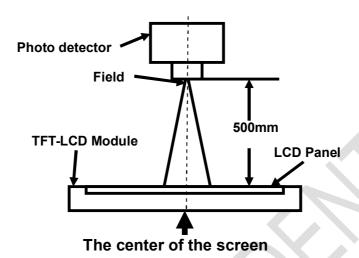
Note 2: Definition of viewing angle range and measurement system. viewing angle is measured at the center point of the LCD by CONOSCOPE(ergo-80).
