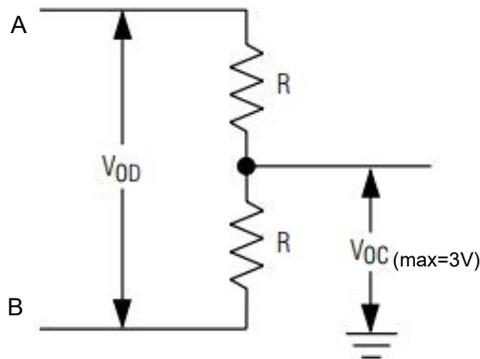
The Matching resistance at both ends of A and B is 120Ω;
